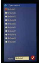
Up to ten pre-set methodologies can be stored in the instrument, easily modified and saved, and can be recalled for repeated use.
