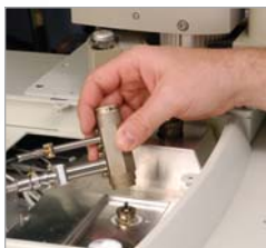
Remove FID cell assembly.
