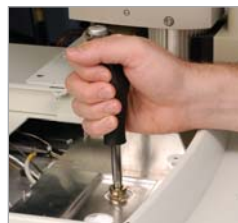
Turn counterclockwise to loosen jet.
