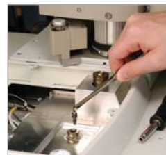
Use tweezers (cat. #20101) to remove jet.
