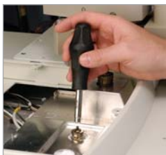
Slip tool over FID jet.
