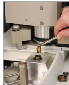
Use tweezers (cat. #20101) to remove liner cap.
