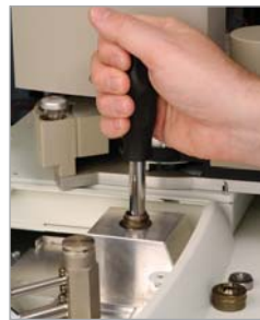
Turn counterclockwise to loosen liner cap.
