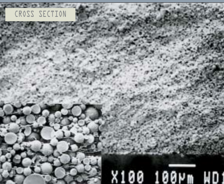
Micrograph of an Empore extraction disk cross-section containing 12µm particles. (inset: 10µm magnification). The smaller particles are the key to more efficient sample preparation.
