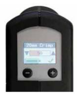
The tool's convenient controls located on the top of the unit allow to adjust the crimp. The OLED screen displays the tool's size, battery status, crimp setting and cycle results. The settings menu provides lifetime statics, recent cycle log, 8 language options and reset functions.
