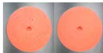
Coated MN septa after exposing to dust and wiping.
