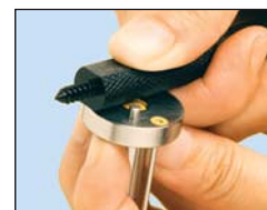
Use the flat side of the Piston Seal Insertion Tool to seat a Waters™ face seal.
